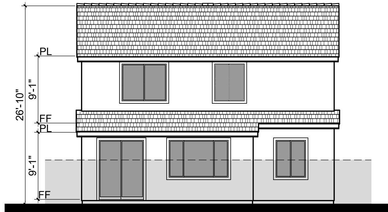
Rear Elevation - 1A Opt. Covered Outdoor Room
