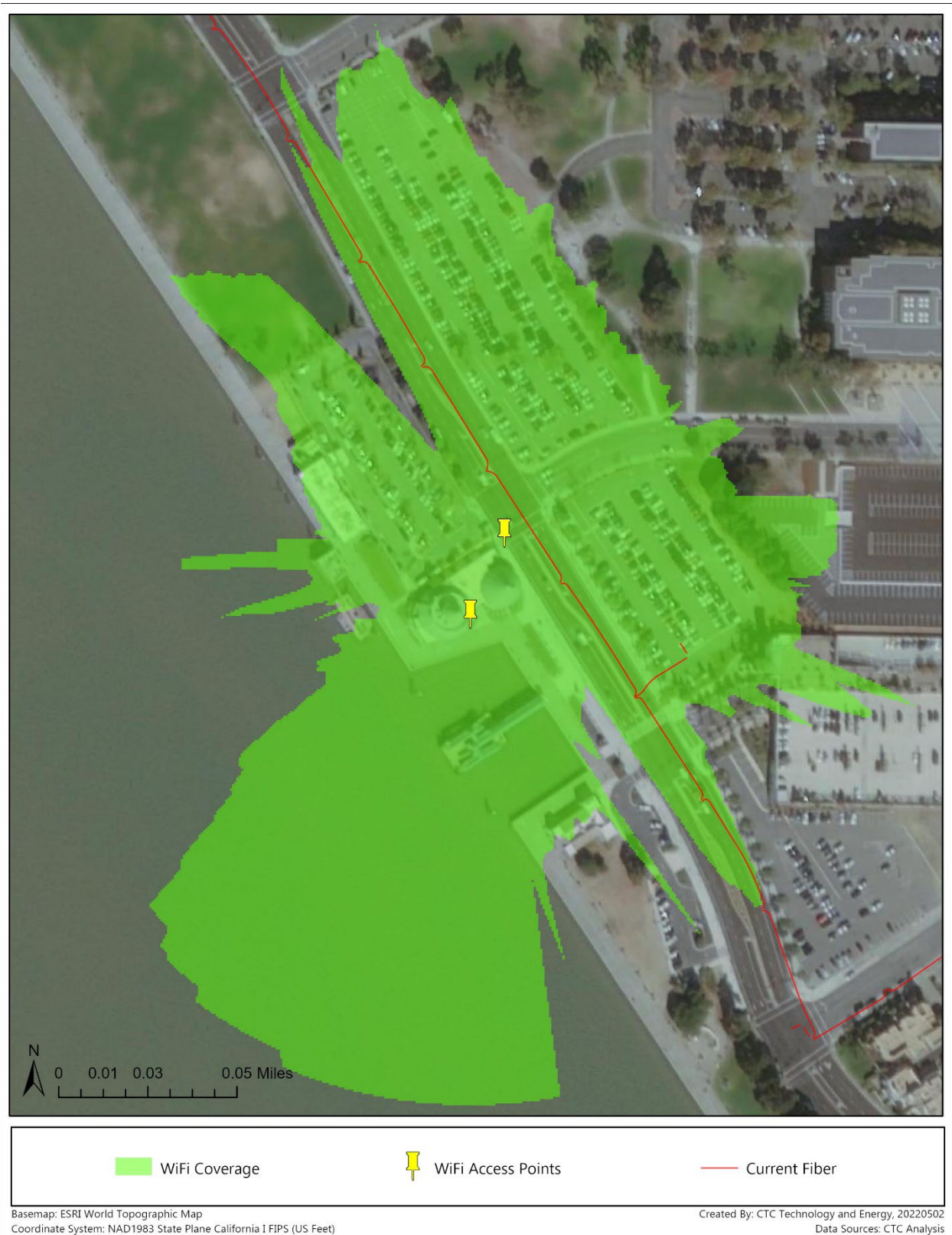
Figure 20: Wi-Fi coverage for Mare Island Dry Dock
