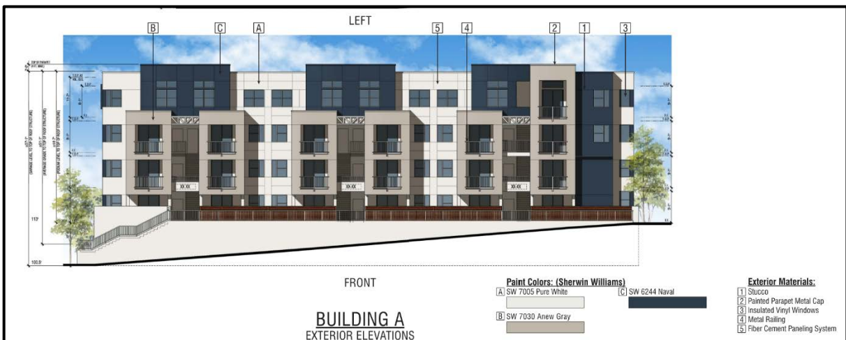
Figure 3 – Building A Elevations
