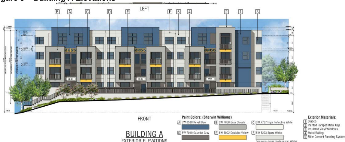
Figure 3 – Building A Elevations
