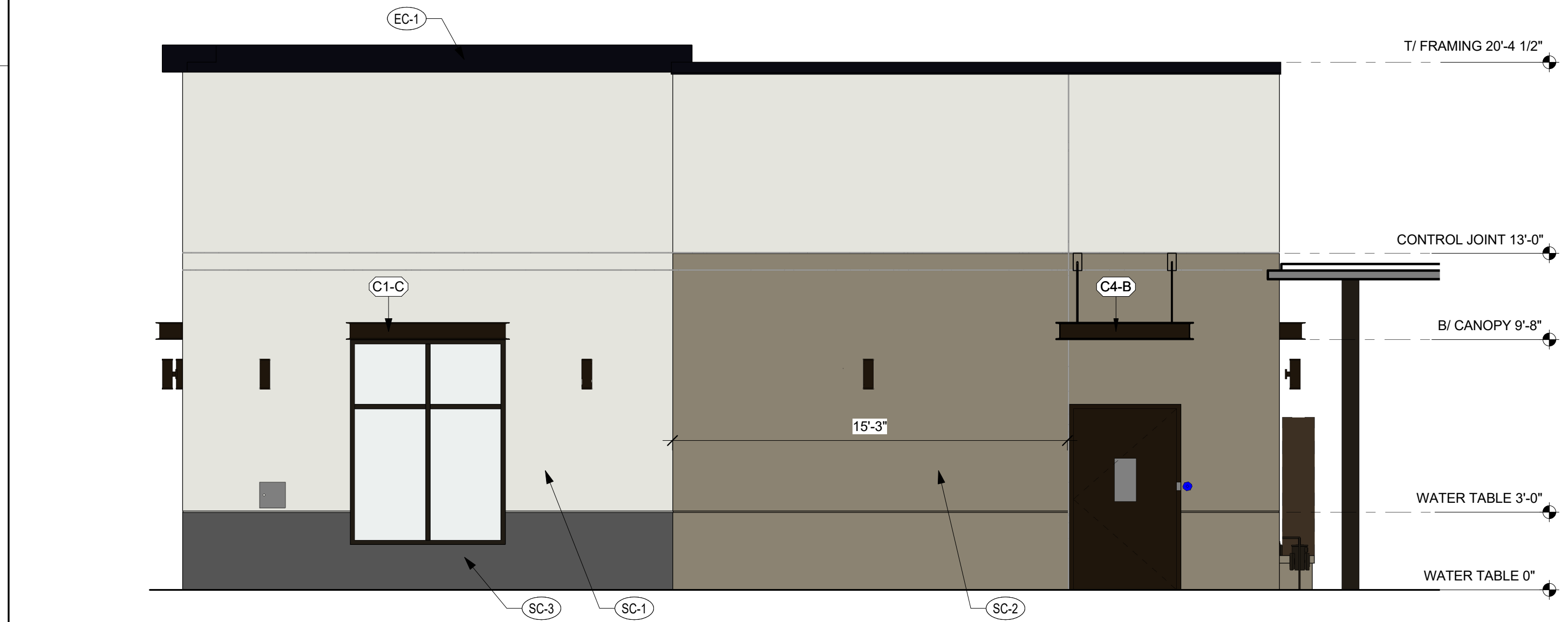
B3 NORTH EXTERIOR ELEVATION 1/4" = 1'-0"
