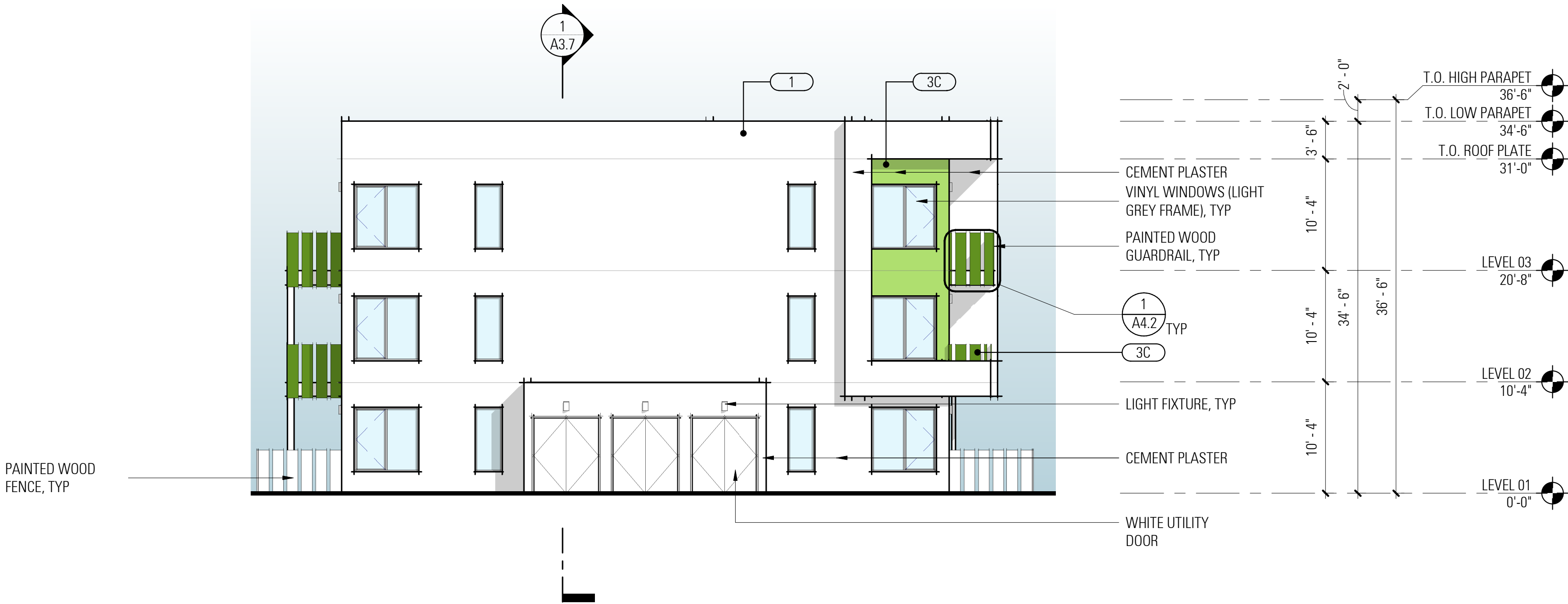
1 A3.2 1/8" = 1'-0" EXTERIOR ELEVATION - NORTH (BLDG TYPE A)
